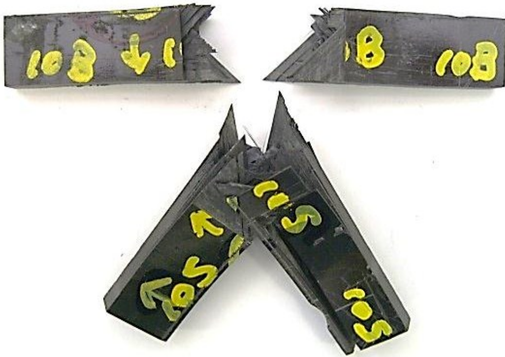
Fig. 3-23 Fracture surface of after impact test
