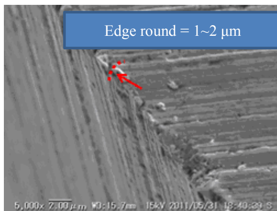
(a) SEM photo by hollow type drill
