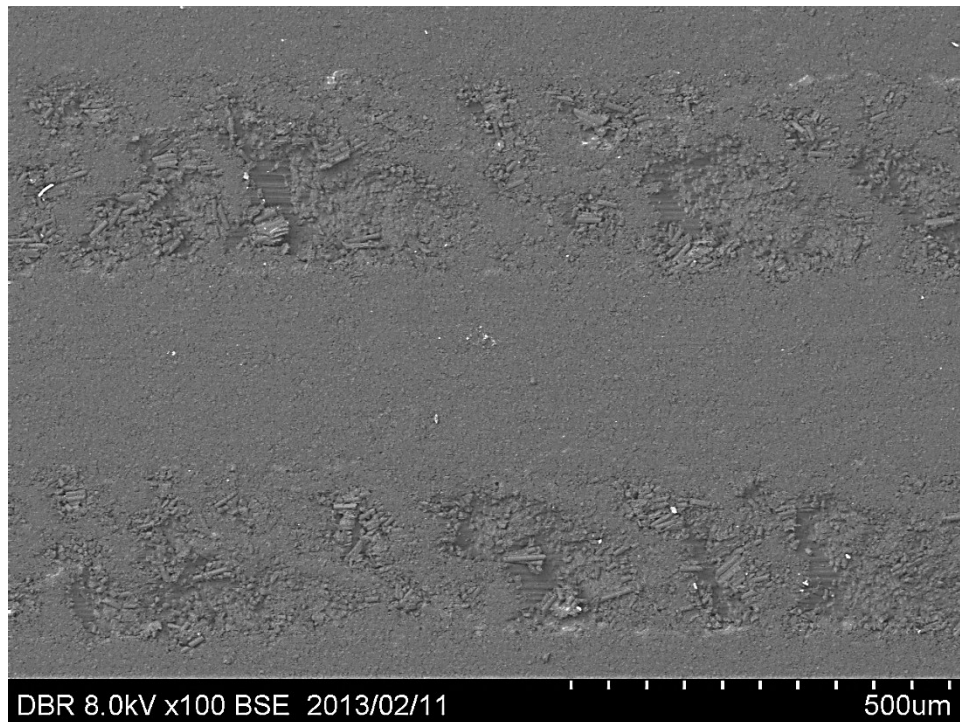
Fig. 2-22 SEM image of finish surface of material C (45°-45°) machined with Tool No. 2 (Helix angle 30°)
