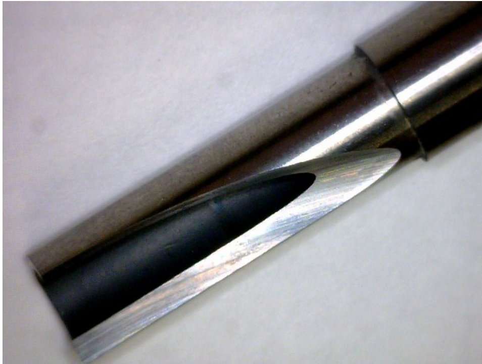
Fig. 5-18 Model 1 prototype hollow type drill
