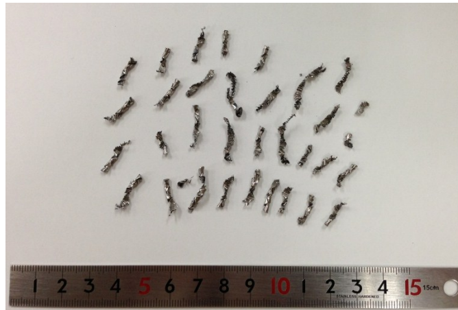
Fig. 4-90 State of Ti alloy cutting chip (M314) (Cutting conditions : Table 4-28 f=0.15\text{mm/rev} )
