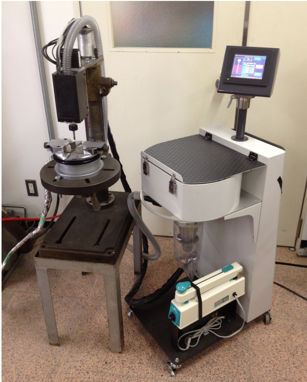
Fig. 5-4 Drilling system (Left) and cyclone type dust-collector (Right)
