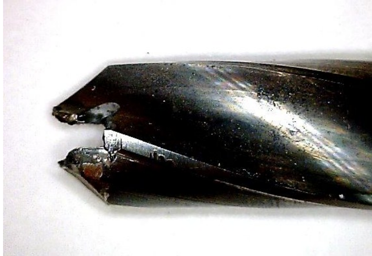
Fig. 4-71 Tool damaged (PCD-GDN)
