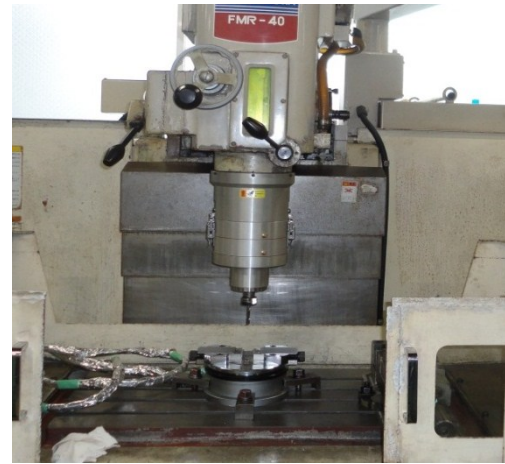
Fig. 4-26 Set up with modulated revolution device
