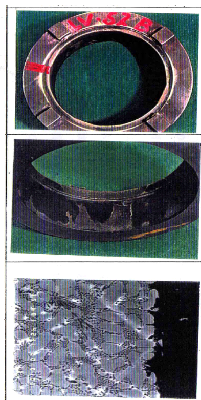
Seat ring of drain level control valve of high pressure heater
