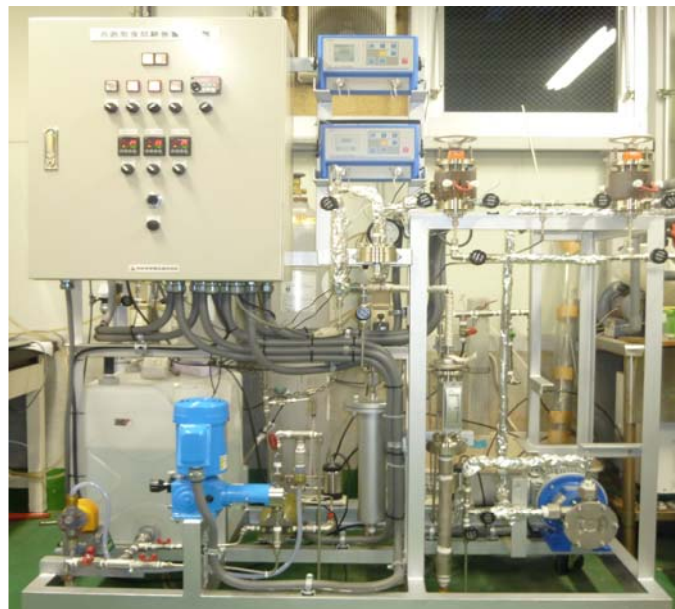
Fig. 4-2 The photograph of Jet-In-Slit testing apparatus for FAC
